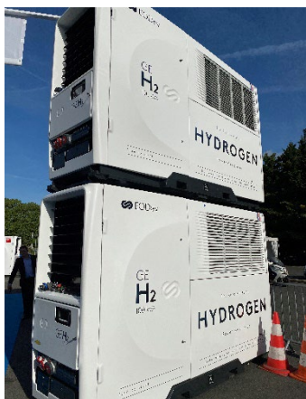
EODev brand generator integrating a PEM Toyota battery (photo B. Blez at the 2023 Hyvolution show)
